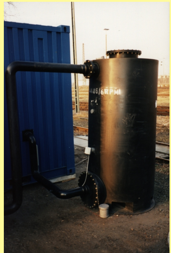
IEG GAC-Sorb™ 1000 System for adsorption of volatile organic compounds
